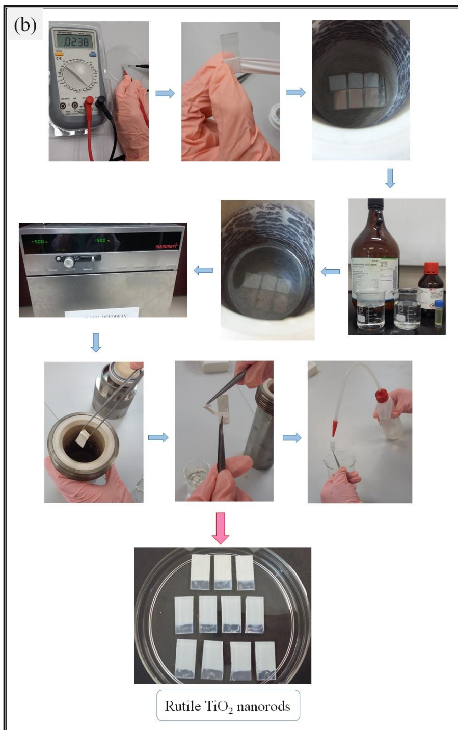
Figure 12. (a) The schematic diagram and (b) experimental procedures to synthesize rutile \text{TiO}_2 nanorods.
